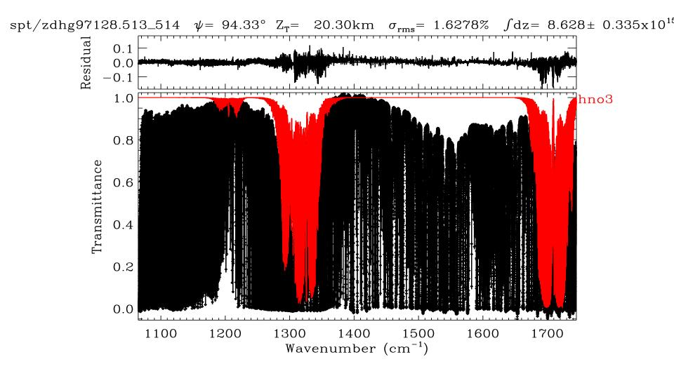
Even using the new MIPAS-1220-1396pre linelist, fits to MKIV balloon spectra in the lower stratosphere (20 km tangent altitude) are still dominated by HNO<sub>3</sub> spectroscopic problems. [With HITRAN\_2012 HNO<sub>3</sub> linelist, residuals around 1300-1350 cm<sup>-1</sup> reached 30%.]
