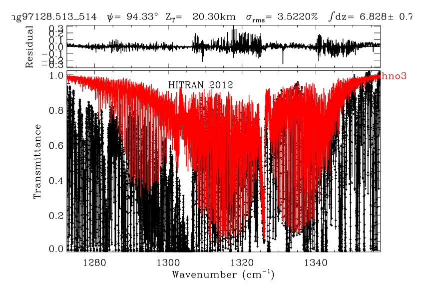
Main absorbers are CH<sub>4</sub>, H<sub>2</sub>O and HNO<sub>3</sub>. Peak residual exceed 30% and the rms is 3.52%
