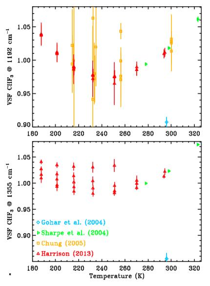
Used the final linelist to retrieve the CHF<sub>3</sub> VMR Scaling Factors from lab spectra. In a perfect world, these would all be 1.0.
