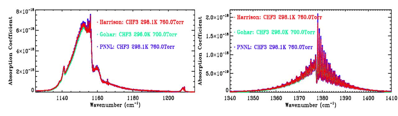
These cross-sections seem fairly consistent. The Gohar cross-section are smaller than the others below 1154 cm<sup>-1</sup>, but very consistent above.
