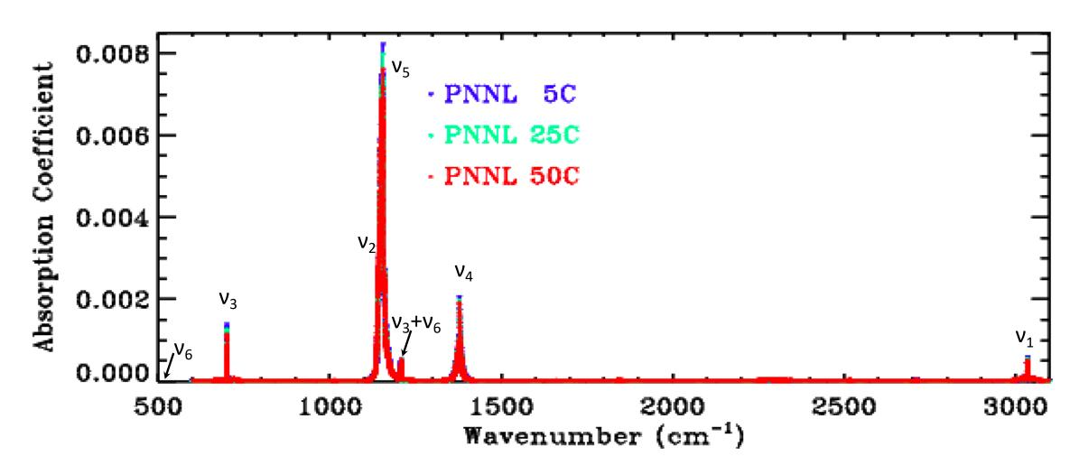
The  $v_5$  bands is the strongest and fortuitously fall in the most transparent windows. PNNL spectra don't cover the  $v_6$  band centered at 508 cm<sup>-1</sup> (Gohar spectrum does). The  $v_3$  band centered at 700 cm<sup>-1</sup> is useless for atmospheric observations since its strong, sharp, Q-branch is overlapped by  $CO_2$
