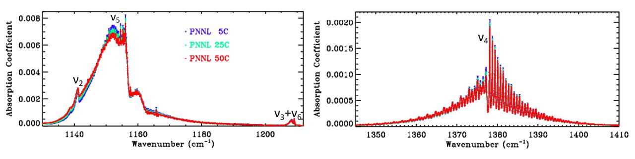
In the band center the absorption coefficient is largest at the cold temperature (blue), implying a low E". In the wings the absorption is largest at high temperature (red) implying high E".
